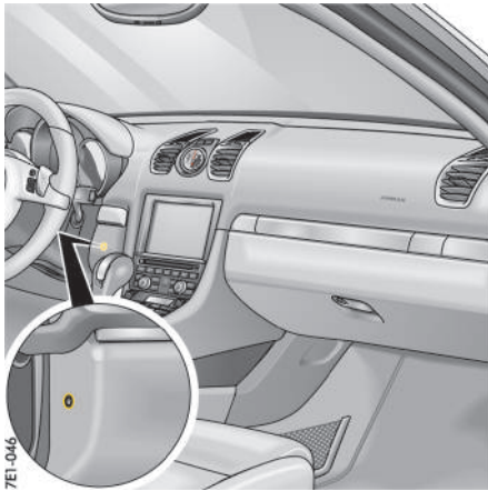
Interior temperature sensor
